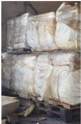
Figure 1: TCCA bags stacked three-pallets high as a precaution from floodwater
