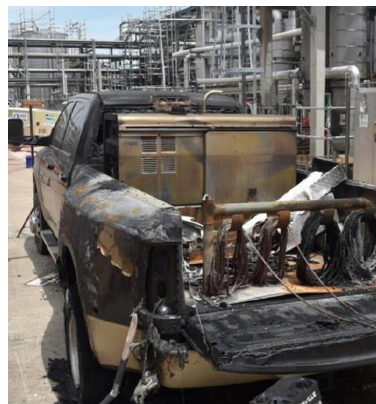
Figure 2: The welding machine on the back of the pickup truck, post-incident
